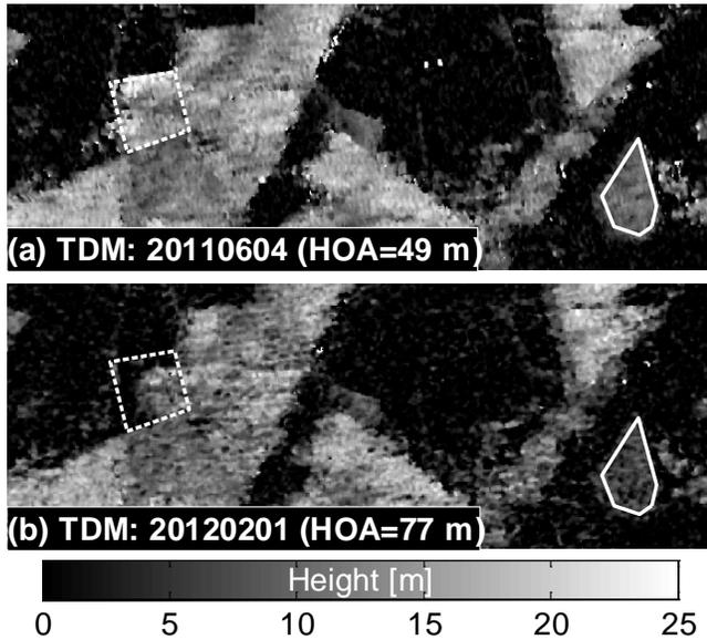
**Figure 4** A comparison between two TDM DCMs for a 1600 m x 600 m region in Remningstorp is here shown. The birch stand discussed in Section 4 is delineated with solid lines. Also, a clear-cut is detected and delineated in dashed lines. VV-polarized TDM data acquired at the nominal angle of incidence of 41° were used for TDM DCM estimation.
