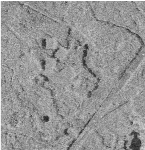
Fig. 5b. TerraSAR-X HH polarized image (look angle \sim 38^\circ ) acquired on 2009-10-07 after the simulated wind-throw.
