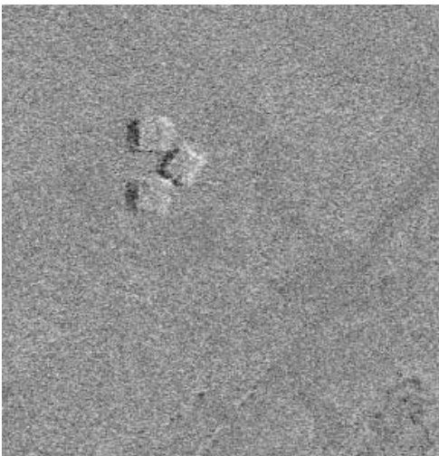
Fig. 5c. Ratio of TerraSAR-X HH polarized images (look angle \sim 38^\circ ) acquired on 2009-10-07 and 2009-09-04.
